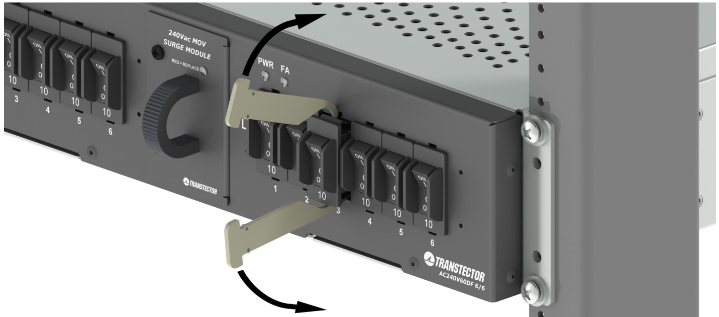
Figure 6: Removing a breaker
